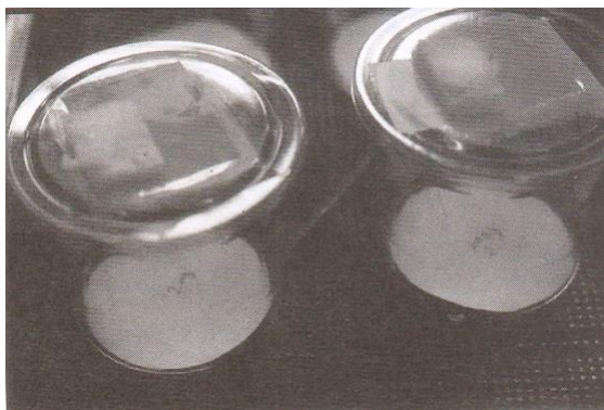
Figure 8. Clear plastic cup used in the experiment. Cut an opening in the center of the lid and attach a net. Stick damp cotton to the top and put filter paper on the bottom.
